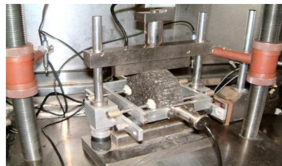
Gambar 1. Indirect Tensile Stiffness Modulus (ITSM) test
