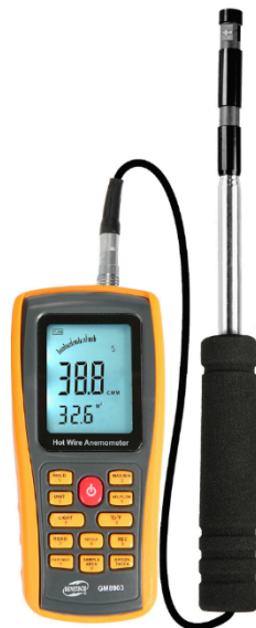
Figure 4-5: Hot Wire Anemometer (GM8903).
