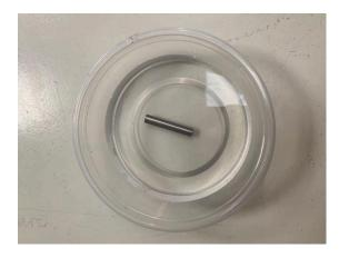
O After leaving the components it to soak for several minutes blow the control valve (in the correct orientation) and the nozzle through with canned air, repeat if necessary
