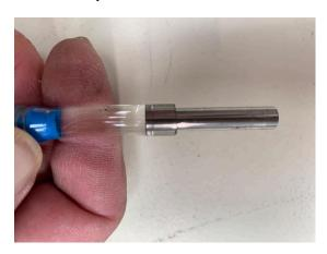
O Separate the control valve and the nozzle from the nozzle holder and place all the components in a bath of specialist herbicide cleaning solution
