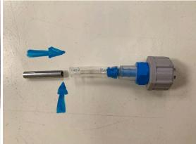
O Gently disconnect the control valve from the sprayer end of the feed tube
