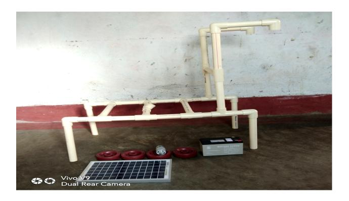
3. Now, the solar plate is fixed by using the structure made with the help of PVC pipes. The motor is fixed using a 1.5 inch CPVC pipe which is clipped using steel clips inverted through the body. The blade is fixed using M- seal to the shaft of the motor.
