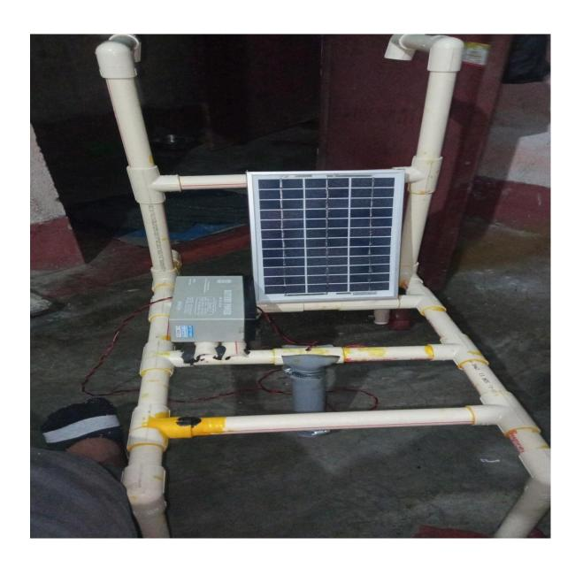
4. The Solar Panel , the battery and the Motor are given connections using the DPDT switch .
