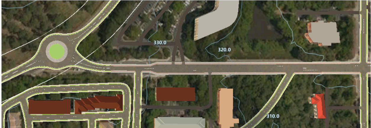
Figure 10: Roundabout model for Alternative 1 (Created via Autodesk InfraWorks)
