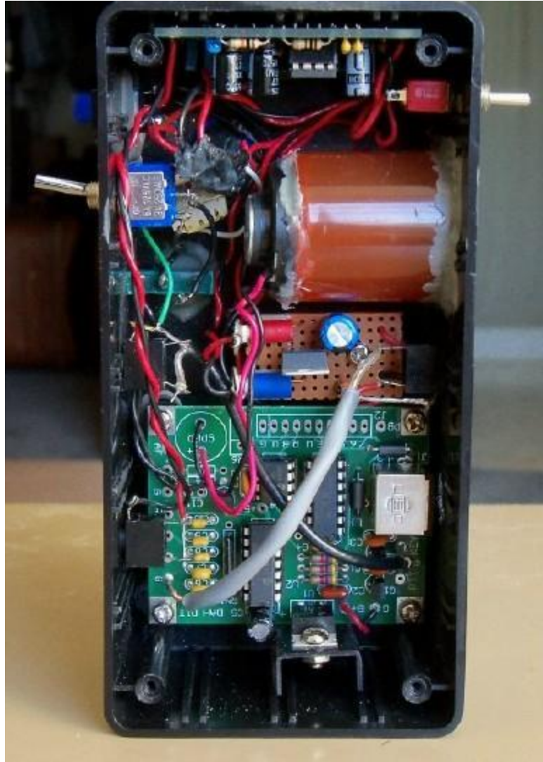
Figure 6. iCW circuitry added to K40 keyer
