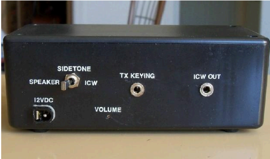
Figure 7. Back view of K40 keyer modified for iCW operation
