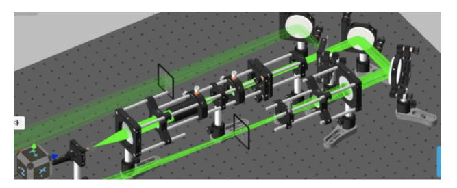
Each optical element is mounted in a plate that has bores for four 6mm ground steel rods that take care of the bulk of coarse alignment. I'd like to be able to mount the laser on this cage system as well for elegance + convenience. The laser mount is one of the 'ends' of the system and emits light through a collimator and onto the grating, which will reflect at roughly a 45° angle (44.60516° to be more accurate) into the next element, similar to one of these:
