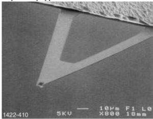
If the laser has been aimed very near the edge of the substrate, slowly moving in "Y", it will cross a maximum of four legs on the two "V" shaped cantilevers.
