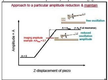
At this point, the amplitude is reduced by 10% relative to its value just beyond the surface, due to onset of tip-sample interaction. Once the Setpoint is reached, the approach stops, the control box beeps, and imaging commences immediately. If engage aborts because the SPM head is still too far from the surface, go back to Stage/Locate Surface and use the trackball to re-locate the surface.
