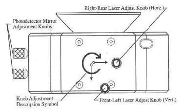
8.4.3 The front-left positioning screw atop the SPM head moves the beam along the Y direction perpendicular to the probe tip cantilever beam. It also moves the laser spot top-to-bottom (vertically) on the photodetector/image monitor. Turning this screw clockwise moves the laser spot to the bottom of the detector screen.
