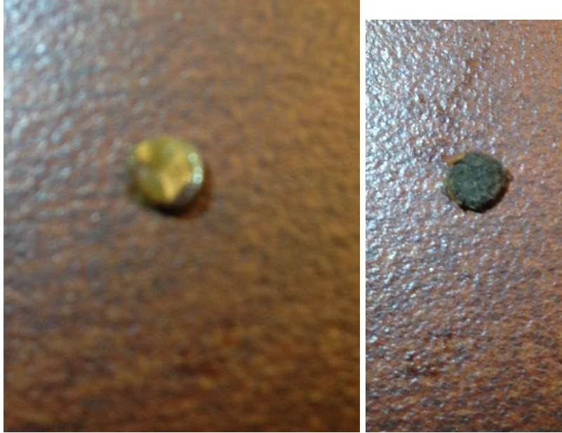
The magnet-coating only remaining on one side
