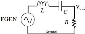
Perform measurements of amplitude and phase to collect enough data to build a Bode diagram for this circuit. Choose a frequency range and number of data points to resolve the resonance peak with enough resolution.
