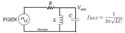
For data collection, choose a span of frequencies so that the resonance peak is well resolved. Make sure there are enough points so that you can identify the -3 dB points (.707 of the peak magnitude) to obtain the circuit Q. Plot the circuit's amplitude and phase response and fit the data to a theoretical (Lorentzian) curve for a resonant circuit.
