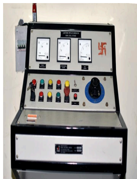
150kV, 225J Impulse Generator Panel
