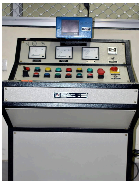
High Voltage 100kV AC DC Test Set Panel
