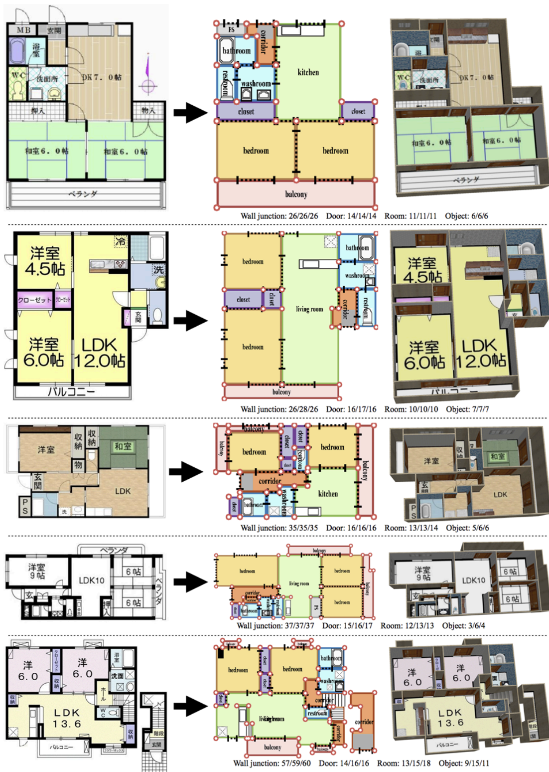
Figure 20: Raster to Vector Floorplan Vectorization Results [2]
