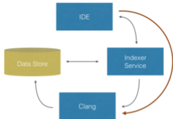
Figure 2. Generating indexing data during a build
