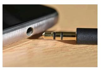
According to a few users, there seem to be inline remote in earphones to enable you to answer calls, change volume, etc. As a result, the earphone jack has a third connector that marries-up with a contact within the phone, in order for the remote functionality to work. This third connector does not make contact with the right internal connection in the phone. To solve this issue, try another earphone of the same type and see if problem persists.
