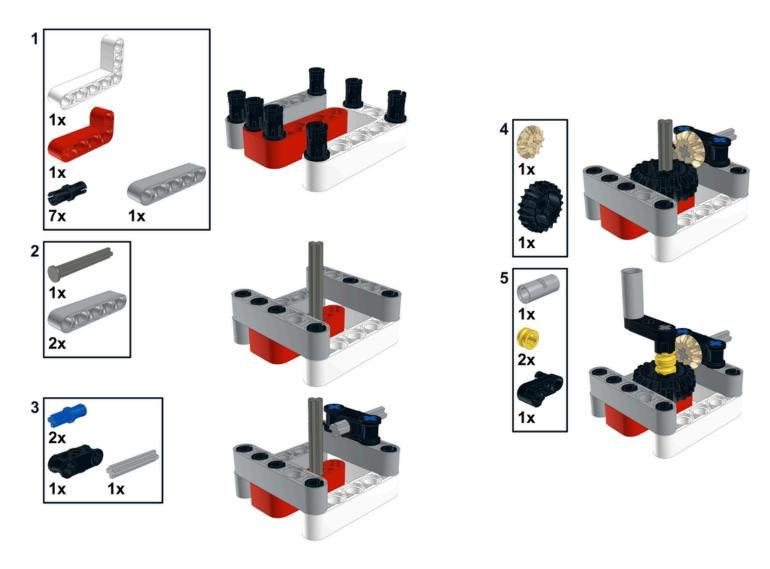
Part 2. Now, let's build the Power Transmission module : Worm gear 8:1
