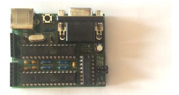
The 'Minimal Terminal' offers a resolution of  $60 \times 25$  characters with each character being displayed as an  $8 \times 8$  pixel matrix and processes the following ANSI control sequences:
