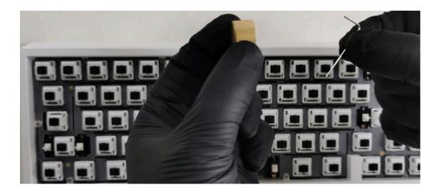
26. Insert the knob hole and tighten the Jim screw in the knob.
