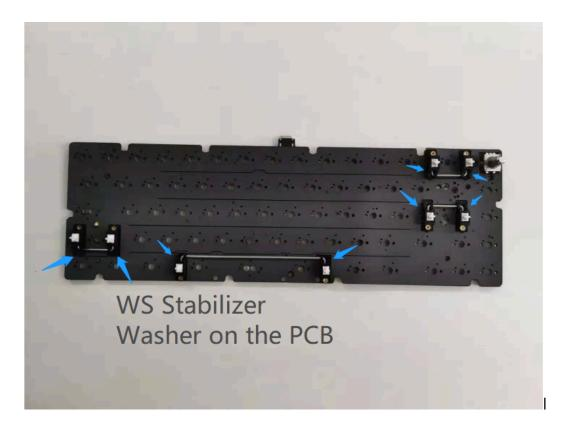
9. This screw is very closed to the switch socket below, please use the small washer under the screw, screw slowly, the washer will bend a little when tightening the screw. This is normal, the hot swap socket is strong enough to absorb the force.
