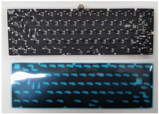
15. Please make sure the holes line up with the PCB foam and take off the **blue film**
