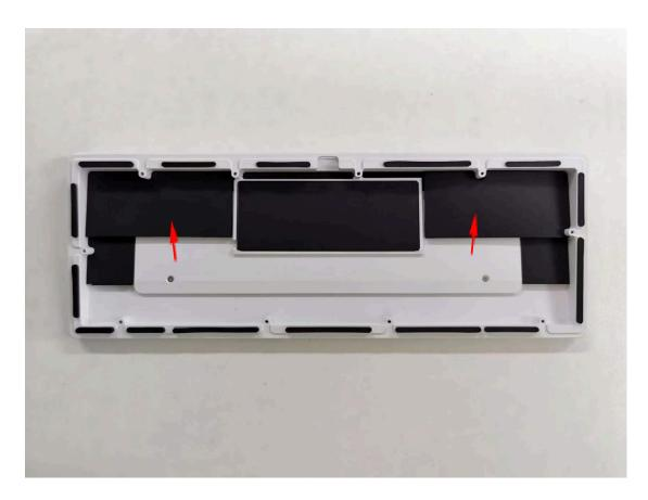
22. Rest the assembled plate + PCB combo on top of the bottom case. Watch out for the positioning of the plate and the screw holes. (Note: plug in the USB port first, make sure it aligns correctly with the USB cutout.)
