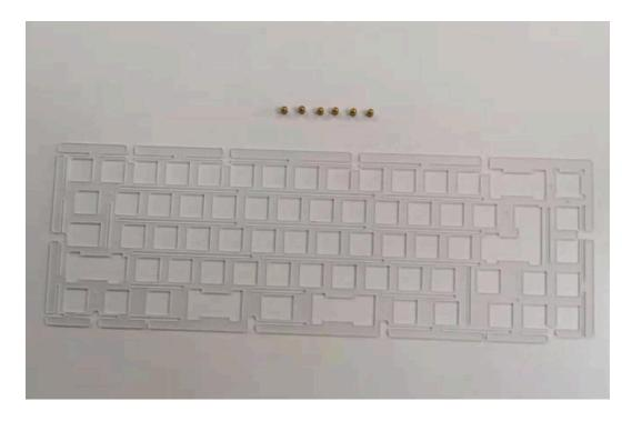
11. Please screw the standoffs on at the back side of the plate(Note: Make sure to screw the red position, otherwise the knob will collapse)
