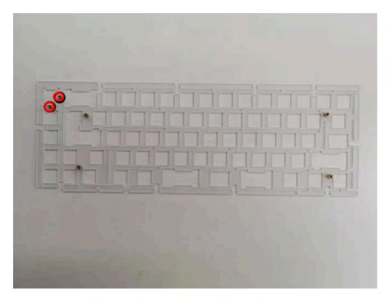
12. Please take out the Plate foam and put it on the backside of the plate. Please be careful and align it well. Mind the positioning of the plate and the standoff holes.
