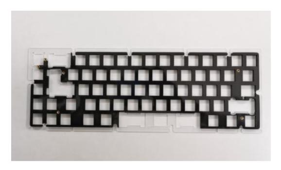
13. Please use the **plastic screws** in the accessory pack to **connect the PCB and the plate** together through the stand.
