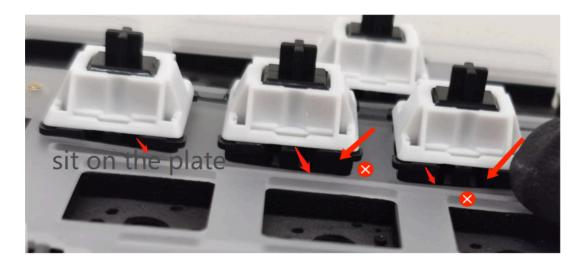
17. Install the switches, and temporarily don't Install the switches at the positions around the case screws as indicated at the of the red circle below
