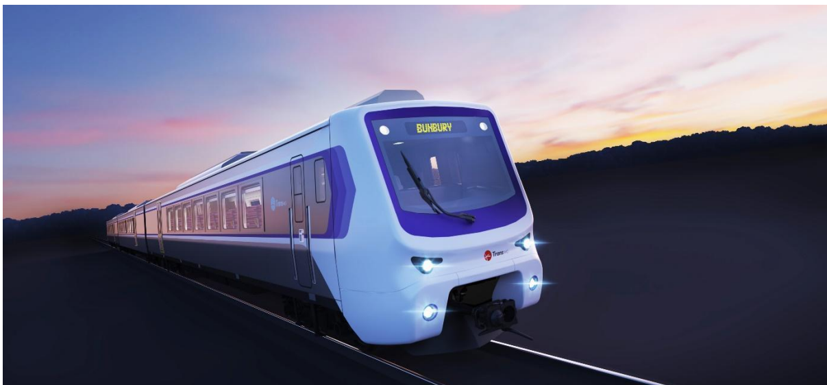
Caption: Artists' impression of the new West Australia regional narrow-gauge trainset. With an operating speed of 130kph, it has a very similar capacity to a Te Huia train-set including seating for 146, with two wheelchair locations expandable to six, an on-board café, space for up to eight bikes, and innovative boarding ramps that address regional station platform-to-train interfaces (image c/o PTA West Australia).
