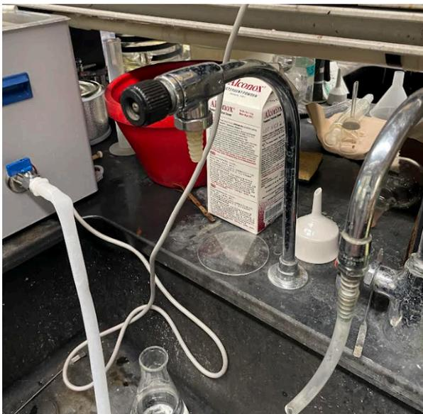
**Deionized water:** DI water is used to clean the pH probe to avoid cross contamination of the solutions. More DI water can be obtained from the sink (see image)
