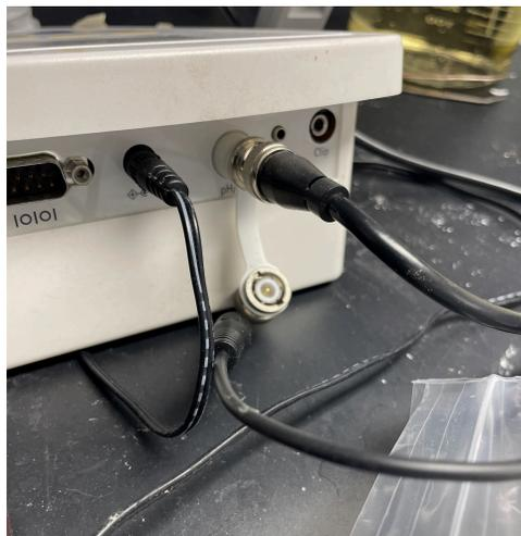
**Ensure that the device is plugged in properly:** The instrument has a power cable that should be plugged into an outlet. In the image, the left thin cable is the power cord. Ensure that the power brick is plugged into an electrical outlet so the device can turn on. The right cable corresponds to the pH probe. Ensure that the probe is plugged in firmly for accurate measurements.
