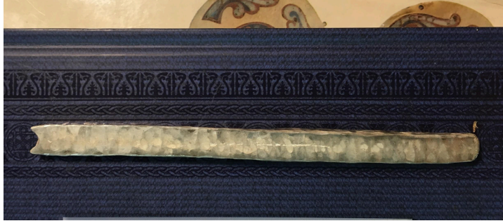
Fig. 27. Forging out the ingot into a square rod, part 2. Source: Marya Kargashina/JessicaSmith-Carlock
