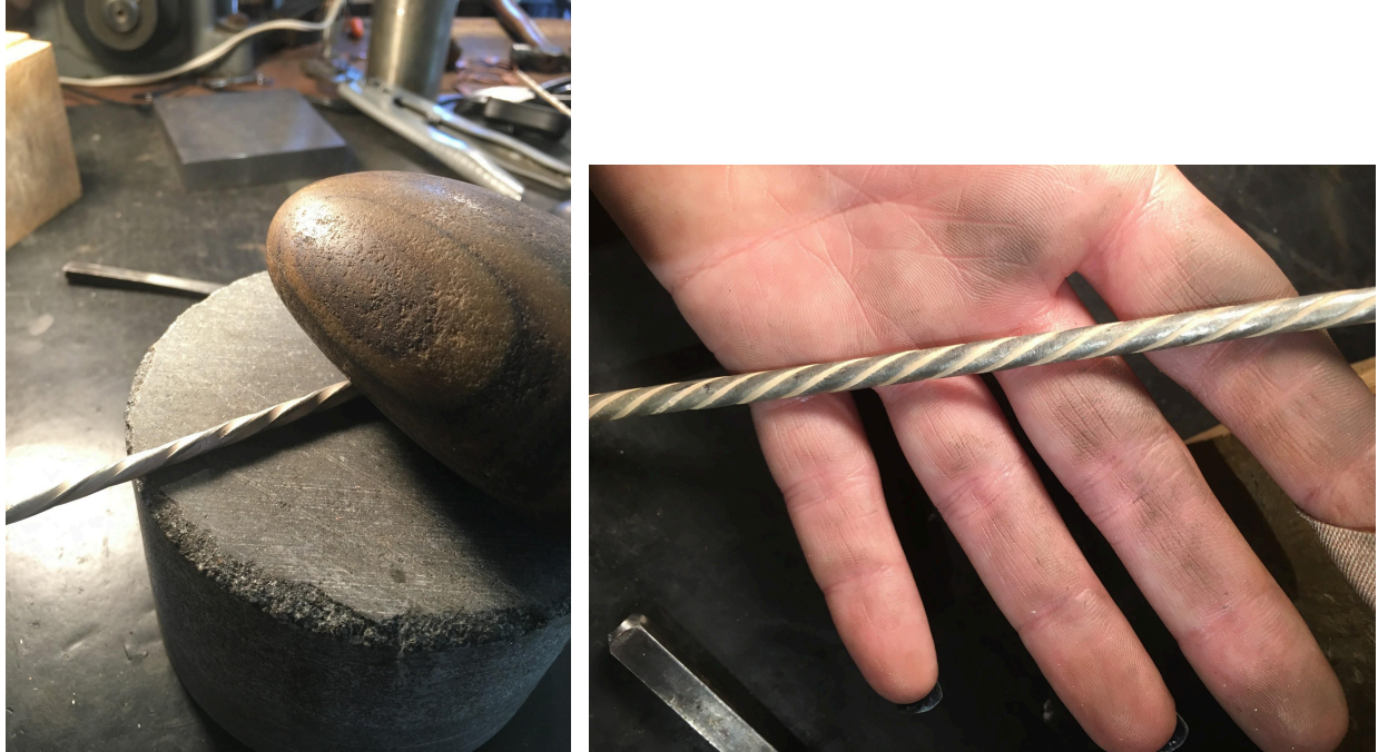
Fig. 30. Smoothing the twisted wire between rocks. Source: Marya Kargashina/JessicaSmith-Carlock
