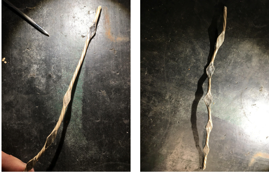
Fig. 32. Starting the flanges.
