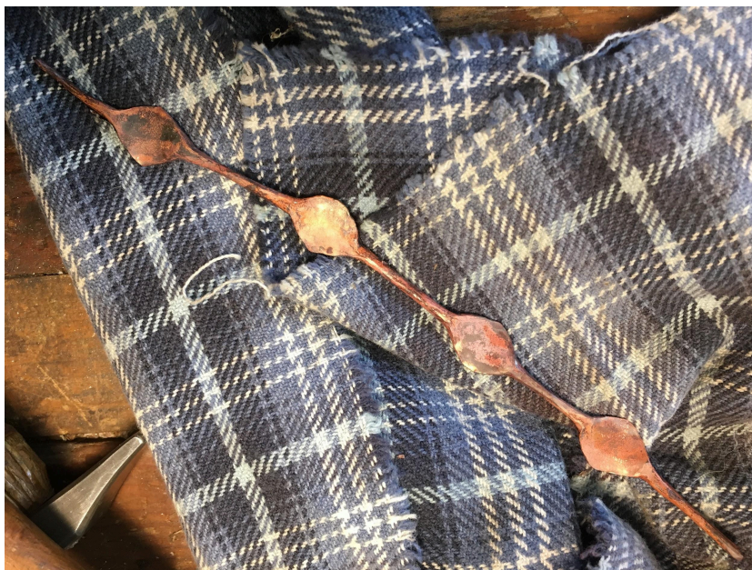
Fig. 22. Twist added between flanges.
