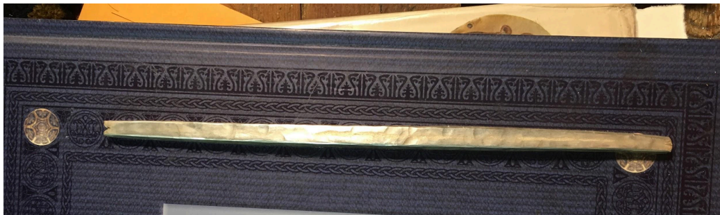
Fig. 28. Forging out the ingot into a square rod, part 3. Source: Marya Kargashina/JessicaSmith-Carlock
