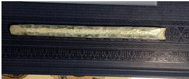
Fig. 26. Forging out the ingot into a square rod, part 1.
