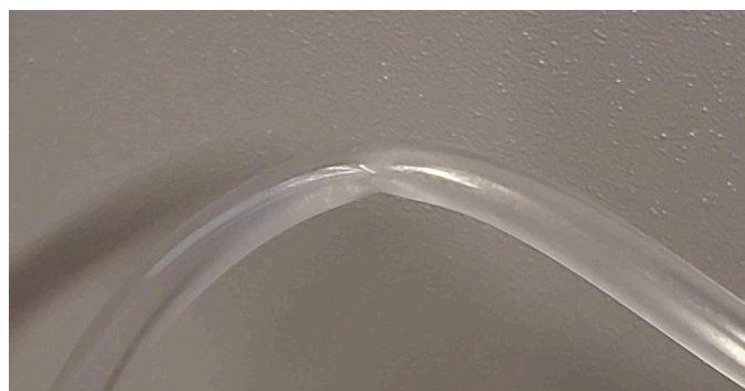
Figure 28. IV tubing after being kinked for 30 seconds.
