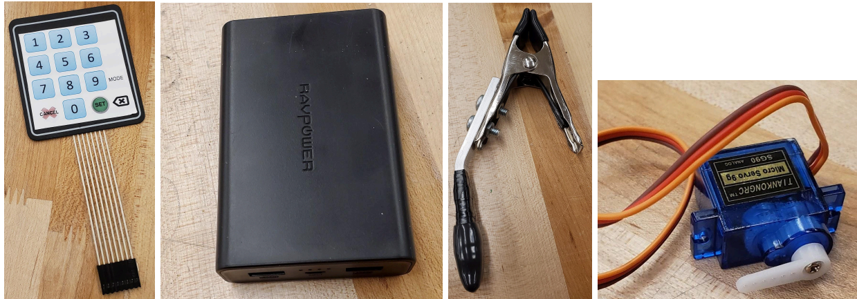
Figure E4. Additional components: left to right: keypad, battery, clamp, servo.
