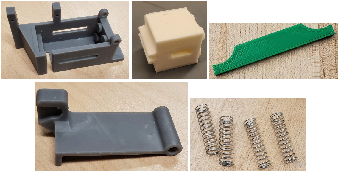
Figure E2. Parts for flow stopper mechanism (left to right and top to bottom): flow stopper wall, slider, puller, latch, springs.
