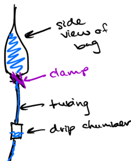
Figure 19. A clamp for the IV bag (rather than the tubing) to control flow rate.
