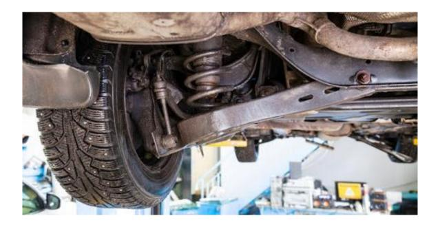
Vibration of higher amplitude and lower frequency are absorbed by suspension spring. Vibration of low amplitude and high frequency are absorbed by the shock absorber.
