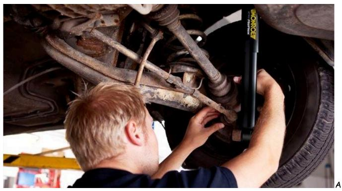
bouncing wheel makes it difficult to control the vehicle and it is to avoid such bouncing of the wheels, a suspension system is provided in the vehicles.
