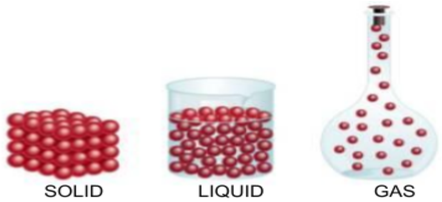
Figure 3. The spacing between the particles in the three states of matter.
