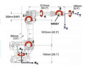
The figure shows a 6-DOF industrial manipulator used in manufacturing. The provided image offers a basic foundation for a comprehensive study of the robot's capabilities and limitations.
