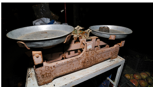
Figure 1.19 A double-pan mechanical balance is used to compare different masses. Usually an object with unknown mass is placed in one pan and objects of known mass are placed in the other pan. When the bar that
