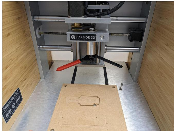
Once the collet is loosened you may remove any tools that may be in the machine (taking care to return them to the correct spot) before inserting your own, this can be done either on the spindle or while the collet is entirely removed like it is shown here
