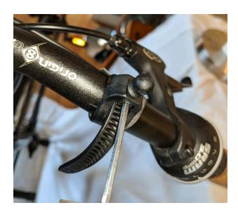
Loosen the small bolt in mirror mount base with the same included allen wrench, so it is open enough to fit around the ball on the handlebar clamp (**first image below**). Pull the base apart and put it over the ball on the handlebar mount and then tighten again (**second image below**).
