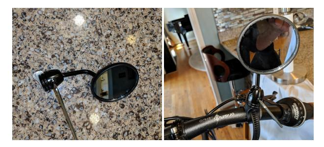
**Note:** You should tighten it enough so you can still move and adjust the mirror, and tight enough to keep it from moving while on the road. You can cut off remaining strap or tape it with electrical tape out of the way.
