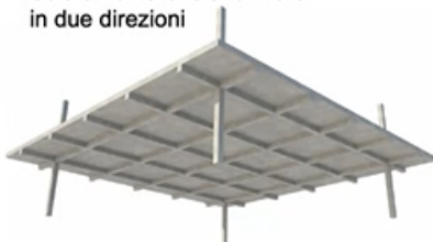
4. Two-way spanning ribbed slab
