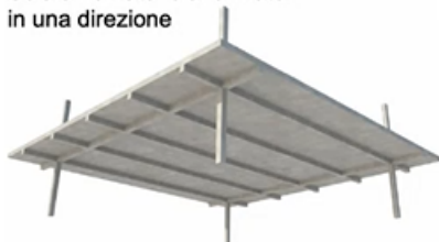
3. One-way spanning ribbed slab
