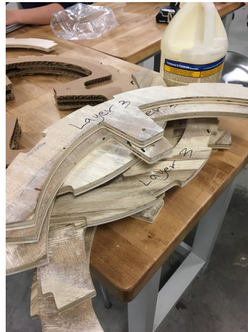
Layer 3 plywood after being sanded.
