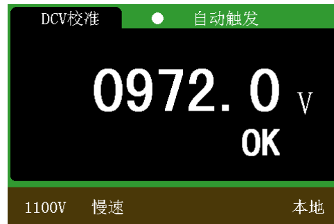
Figure 82 DC voltage calibration is completed
