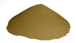
BR 201 Bronze powder is a copper-tin based material, blended and typically formulated to 90% copper and 10% tin. These pre-mixed powders are engineered for low noise sintered bearings. The sintered pore structure of the bearings provides a uniform controlled porosity and oil permeability for excellent hydrodynamic lubrication at lower shaft loads and higher rotational speeds.
