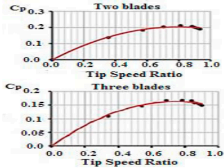
Figure 1-14: The C_p variation with the TSR for two & three blades.
