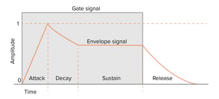
After the filter the sound passed through an amplifier that is controlled by the volume envelope.
