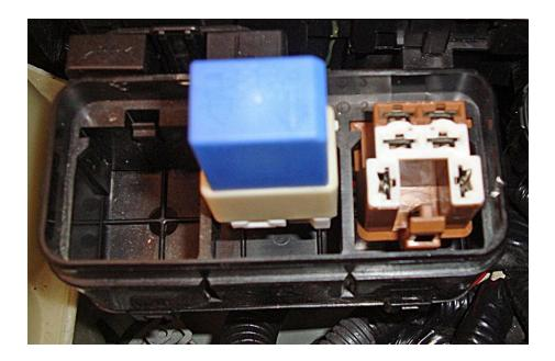
I believe I need the connector to activate the brown towing relay on the right above.
