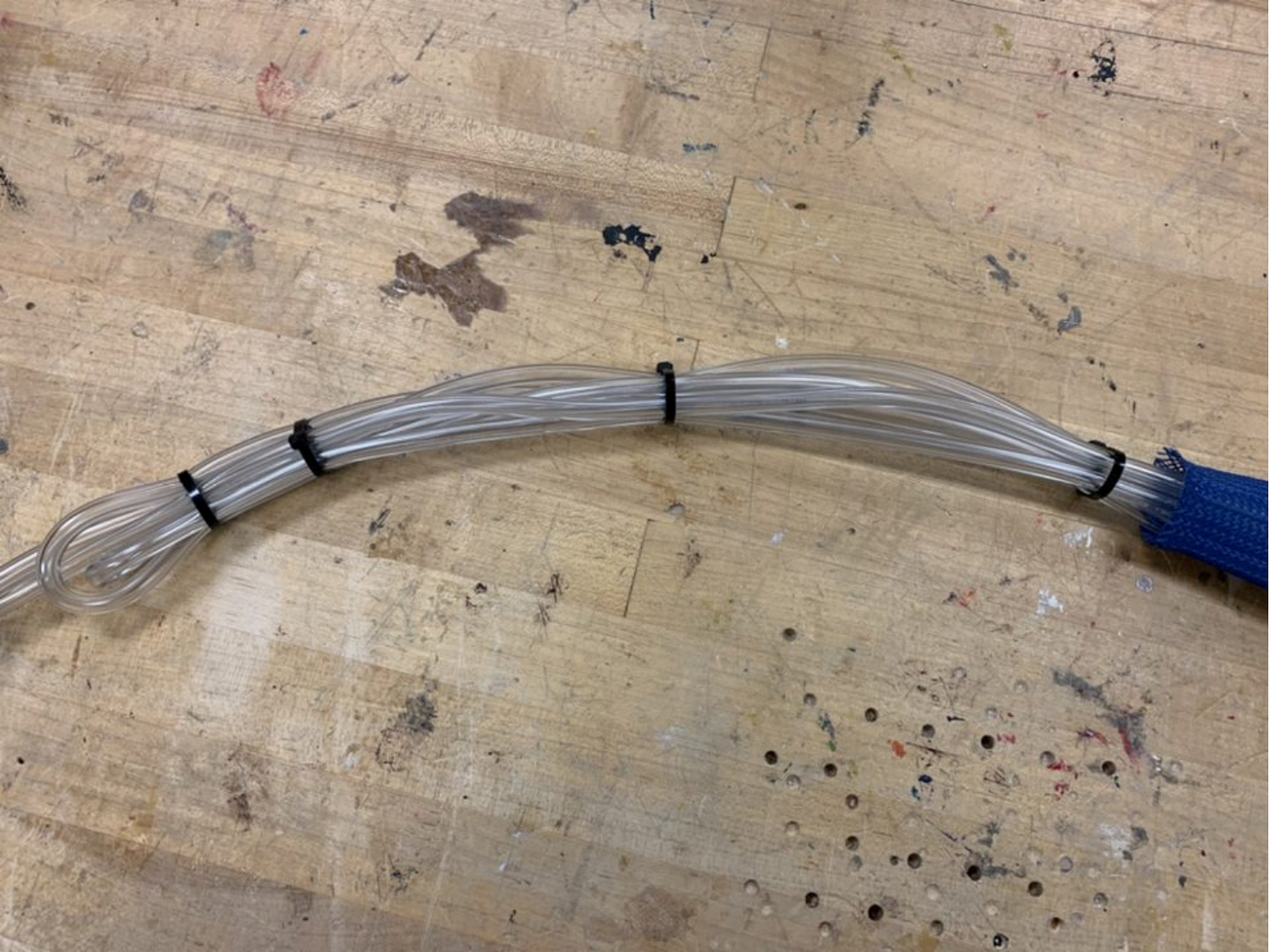
Figure 1: Single pneumatic tube folded over and secured with zip ties to make lifting tube
