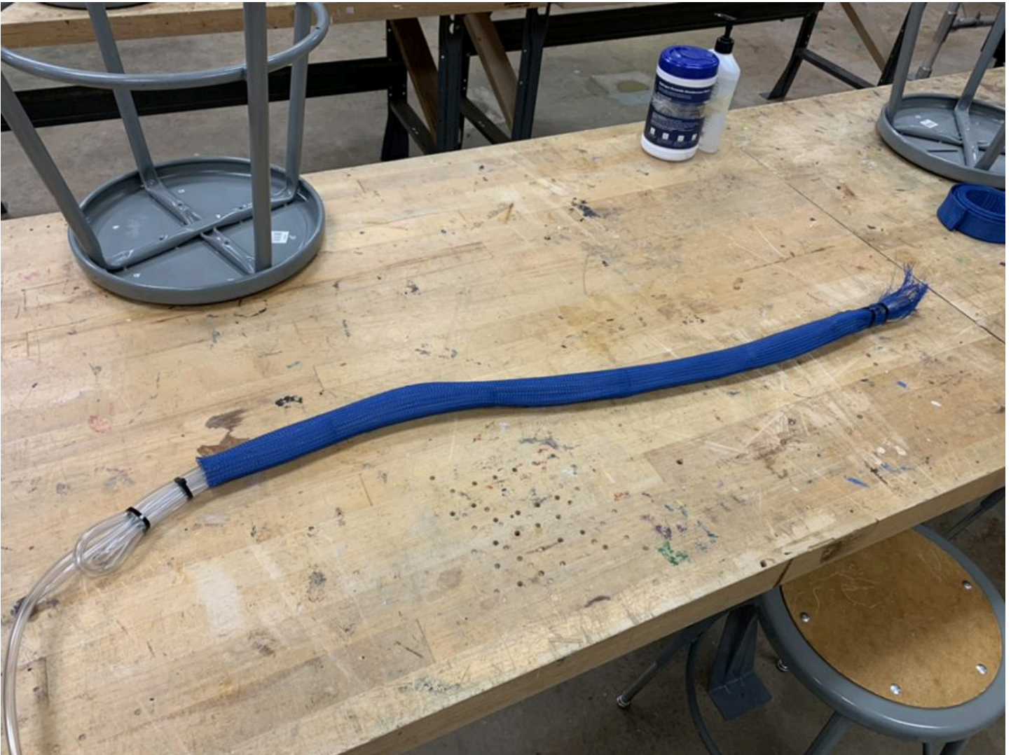
Figure 2: Air tube assembly inserted into nylon sleeve.
