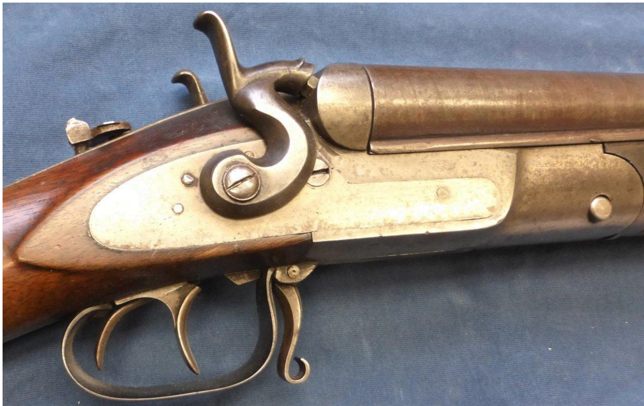
Drilling conversion using Baker's 1875 patent, likely of a Marathon gun; .705" over .400
