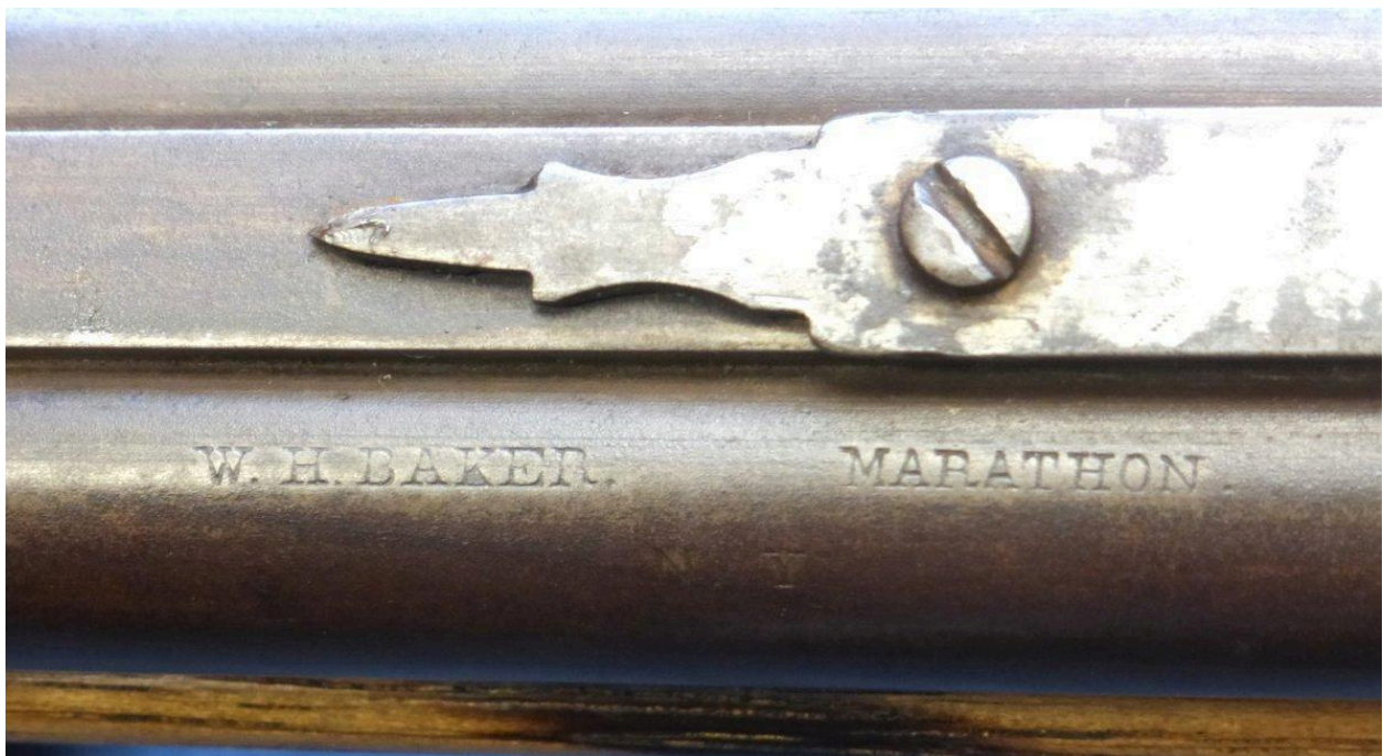
Drilling .354" rifle over .658" shotgun, 29 1/2" barrels
