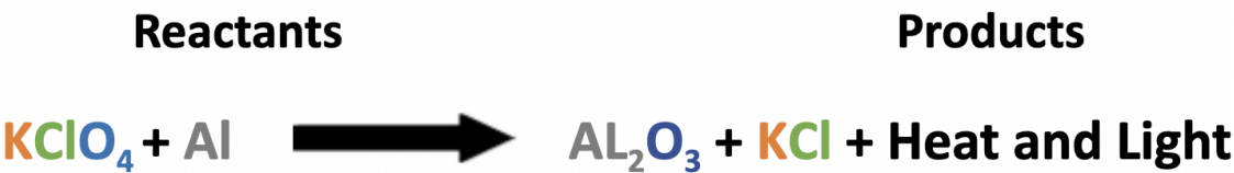
Figure 2: Chemical reaction of fireworks
