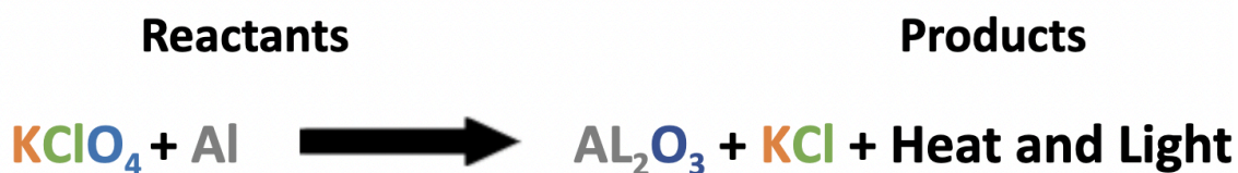
Figure 2: Chemical reaction of fireworks
