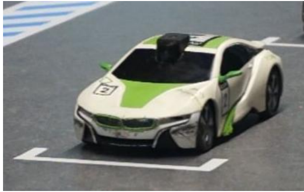
Figure 1: Remote-controlled car equipped with a camera and Wi-Fi connection.
