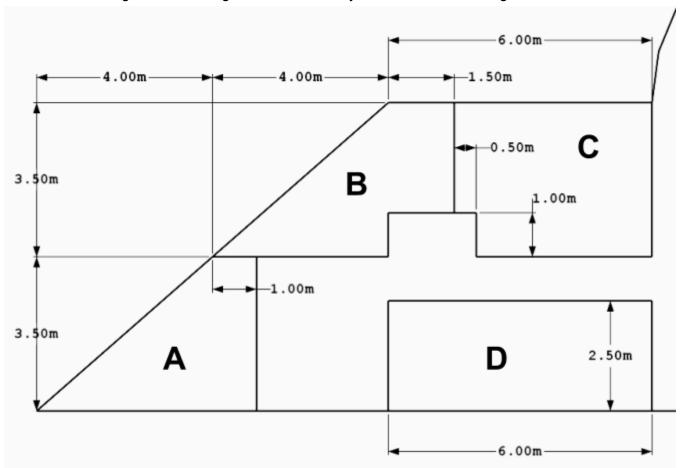
Determine the size of the each room and fill in the sizes at the bottom of the page. (4K, 3T, 2C)
