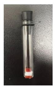
Sample 2: Silicone top layer, teflon spacer, silicone bottom layer (silicone layers are thinner than in sample 1)
