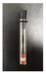
Sample 1: Silicone top layer, teflon spacer, silicone bottom layer
