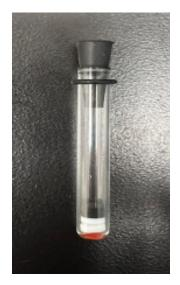
Sample 3: Buna-N top layer, teflon spacer, silicone bottom layer
