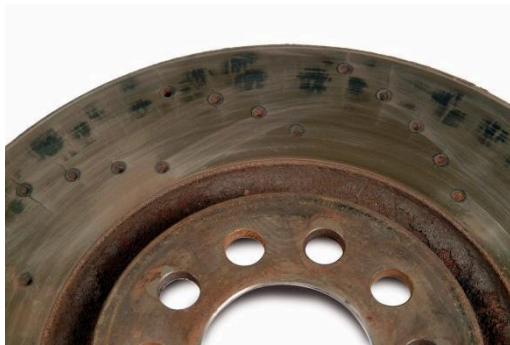
Picture 1: The brake disc shows hotspots due to thermal overload - here easily recognizable by the dark spots.
