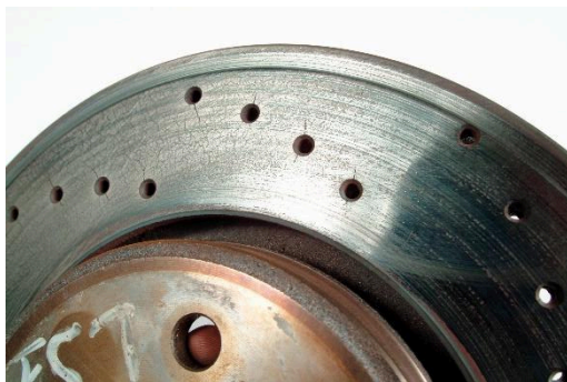
Picture 2: Small, net-like hairline cracks in the disc are not a problem
