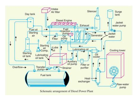
A generating station in which diesel engine is used as the prime mover for the generation of electrical energy is known as diesel power station.
