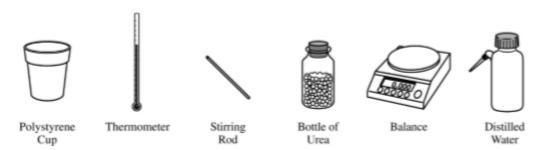
(e) The equipment shown above is provided so that the student can determine the value of the molar heat of solution for urea. Knowing that the specific heat of the solution is 4.18 J/(g·°C), list the specific measurements that are required to be made during the experiment.
