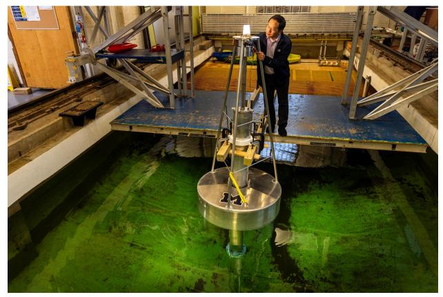
Zuo and buoy.jpg: Inside the University of Michigan's Marine Hydrodynamics Laboratory, Lei Zuo, the Herbert C. Sadler Collegiate Professor of Engineering and a professor of naval architecture and marine engineering, inspects a prototype buoy that generates electricity from wave motion. Whenever the buoy bobs up or down, the light blinks on. Photo credit: Marcin Szczepanski, Michigan Engineering.
