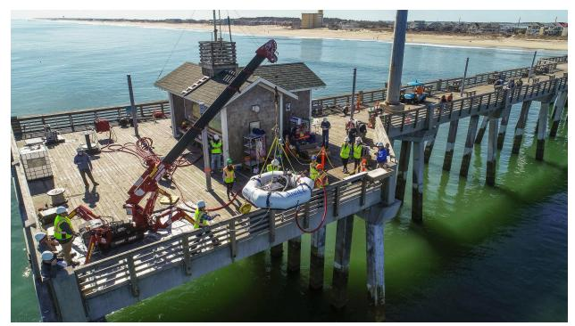
Jennettes Pier Test Deployment.jpg: Jennette's Pier is home to the Coastal Studies Institute's Wave Energy Test Center. The facility has been a testing location for several prototype wave energy devices, such as the National Renewable Energy Laboratory's HERO wave energy converter—the device hanging from the crane. It was built to remove salt from water using wave power. Photo credit: John McCord, Coastal Studies Institute, East Carolina University.
