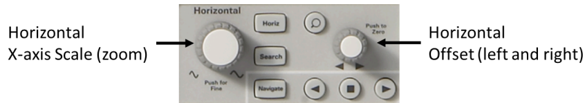
Figure 39: The oscilloscope horizontal x-axis controls
