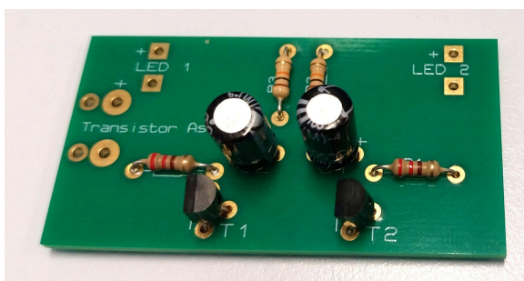
Figure 49: Putting and soldering capacitors on the board.
