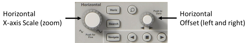
Figure 43: The oscilloscope horizontal x-axis controls
