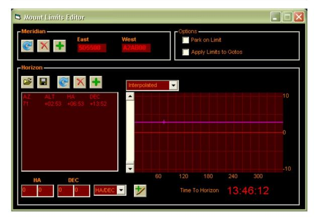
There are two algorithms that determine how EQASCOM uses the points list to calculate an Altitude limit.
