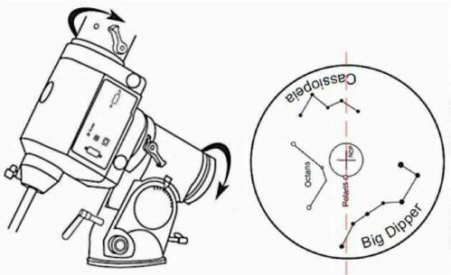
8. Now slew the mount in RA until the Pole Star indicator (the little circle) is superimposed over the Pole Star
