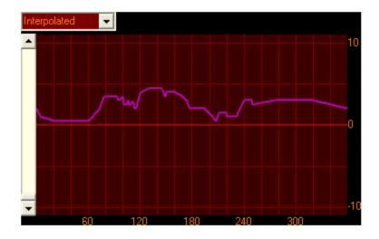
Using "Greatest Alt" mode EQACOM finds the two points on either side of the scopes current Azimuth and uses the one that has the greatest Altitude.
