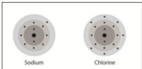
Chlorine's attraction for an electron in sodium is stronger than sodium's attraction for an electron in chlorine. An electron is transferred to chlorine which makes chlorine a negative ion. Since sodium lost an electron, it becomes a positive ion. Positive and negative ions attract and form an ionic bond.
