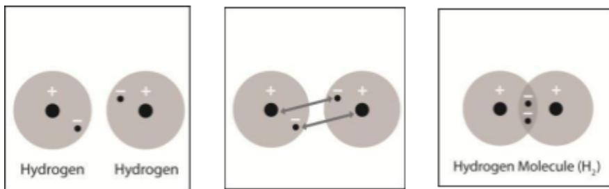
The electron in each atom is attracted to its own proton (not shown by an arrow) and is also attracted to the proton in the other atom (shown by arrows). These attractions bring the atoms together.
