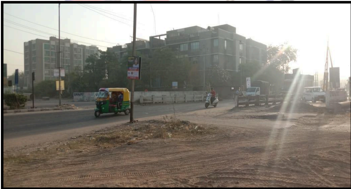
Figure 21 Shoulder width is not provided, full length fences are not provided and huge area under land acquisition reducing road width
