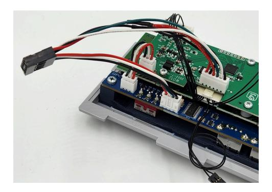
**6.** Plug the USB harness into the motherboard USB header, paying attention to the connector's polarizing key. Plug the reset button connector into the motherboard front panel header, referring to the motherboard manual for its pinout.
