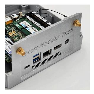
**4.** Plug the USB Type-A adapter board into the first USB port on the motherboard.
