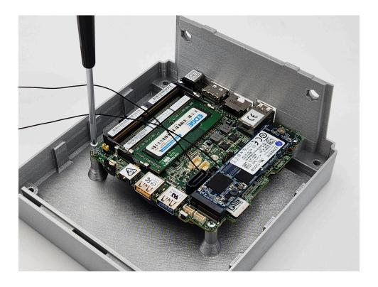
**Installing Wireless Antennas:** If the motherboard is equipped with a wireless module, mount the SMA connectors to the rear I/O shield using a small adjustable wrench.
