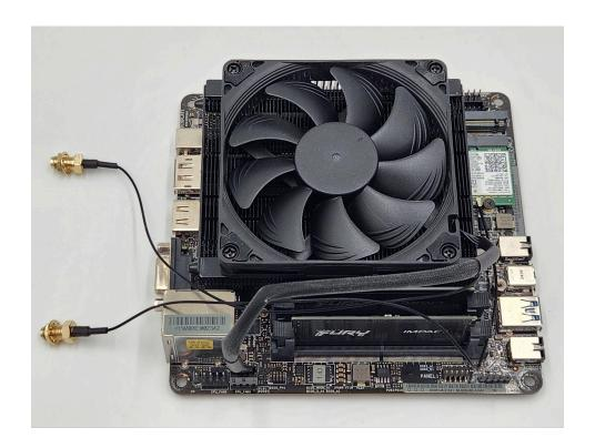
**NOTE:** For Intel models, the CPU cooler backplate may need to be trimmed to fit around the motherboard heatsink.
