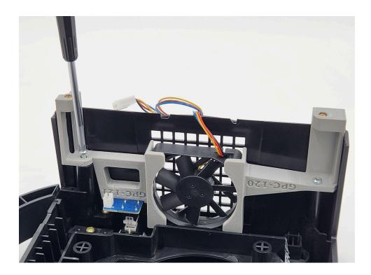
**9.** Place the power button standoff assembly inside the top shell and secure using (x2) M3 x 8mm thread-forming screws, tightening carefully.
