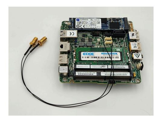
**3.** Lower the motherboard onto the motherboard mount standoffs and push it towards the rear of the case. Secure using (x4) M3 x 8mm screws, tightening carefully.
