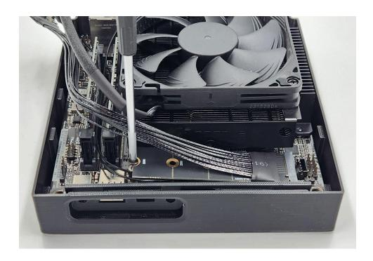
**NOTE:** Slightly loosen the two bracket screws underneath the extension. Adjust the brackets by pushing the OCuLink port board into its cutout. While holding the brackets in place, re-tighten the screws underneath. Secure the extension using (x2) M3 x 6mm flat head screws.
