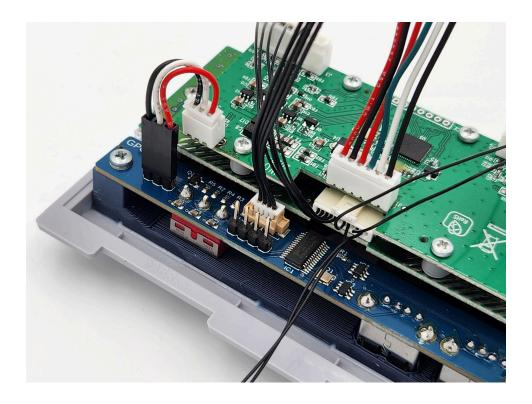
**8.** Set the front panel into the groove in the bottom shell. Plug the USB harness for the controller adapter into the USB Type-A adapter board.
