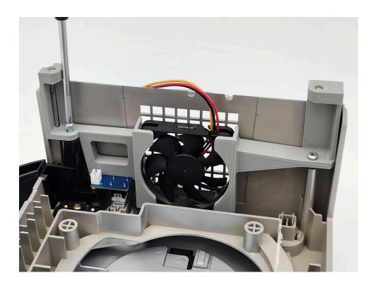
**12.** Secure the power button standoff assembly inside the top shell using (x2) M3 x 8mm thread-forming screws, tightening carefully.
