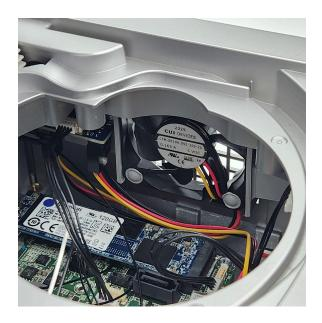
**20.** Secure the top shell to the bottom shell using (x4) M4 x 20mm bolts and (x4) rubber bumpers with the included 3mm hex key. Do not overtighten; the rubber bumpers should only be slightly compressed.
