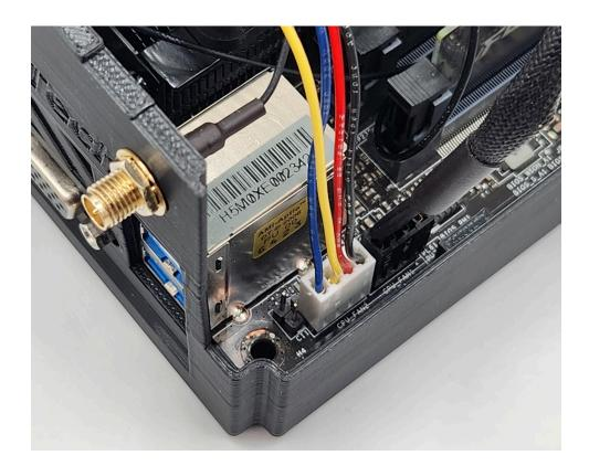
For Motherboards with 1 Fan Header: Plug the fan hub wire harness into the CPU fan header on the motherboard. Plug the CPU cooler fan into the fan hub board's "CPU" header.
