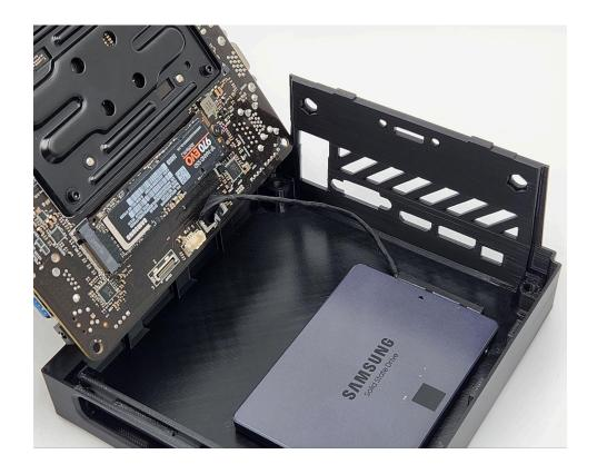
**3.** Angle and lower the assembled motherboard into the bottom shell until it is resting on all four standoffs.
