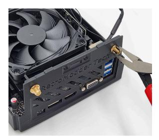
**Installing an OCuLink Interface:** Insert the M.2-to-OCuLink extension in a top-side M.2 slot.
