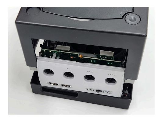
**15.** With the top lid open, slowly slide the top shell down while ensuring that no wires are being pulled on.
