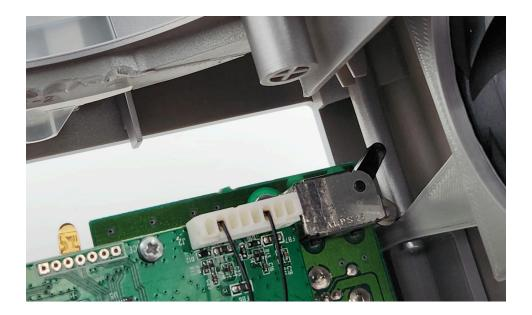
**18.** Ensure that the top shell is fully seated in the bottom shell around the perimeter.
