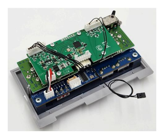
**5.** Plug the USB harness into the 6-pin USB controller adapter and 4-pin USB hub headers.
