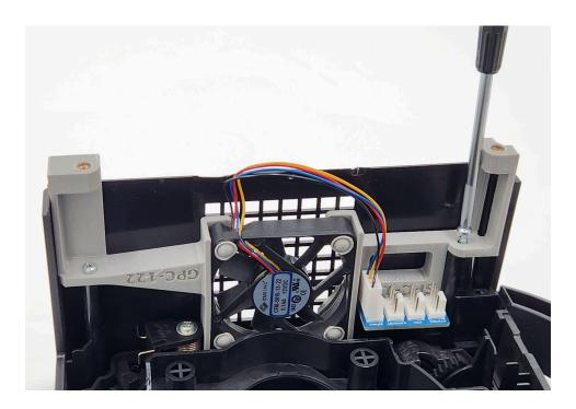
**10.** Plug the intake and exhaust fan connectors into the "INT" and "EXH" headers on the fan hub board, respectively.
