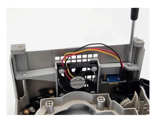
**13.** Plug the intake and exhaust fan connectors into the "INT" and "EXH" headers on the fan hub board, respectively. Plug the fan hub harness into the 5-pin fan hub header.
