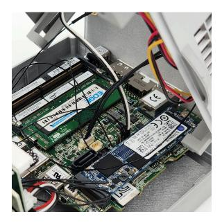
**15.** Plug the fan hub wire harness into the motherboard SATA power connector.
