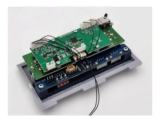
**6.** Plug the USB harness for the controller adapter into the 6-pin USB controller adapter header. Plug the mode switch harness into the 3-pin headers on the USB controller adapter and USB hub board.
