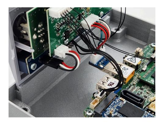
**10.** Plug the reset button connector into the motherboard front panel header, referring to the motherboard manual for pinout.
