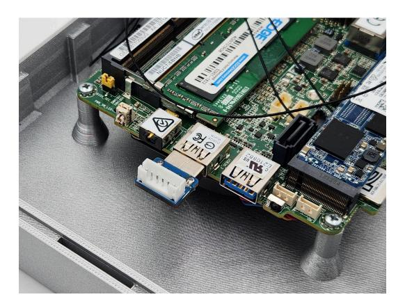
**5.** Plug the controller adapter harness into the controller port board, paying attention to the 8-pin connectors as they are populated differently.
