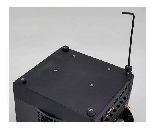
**NOTE:** Use a small screwdriver or the included 3mm hex key to align the threaded hole if the bolts do not thread in.
