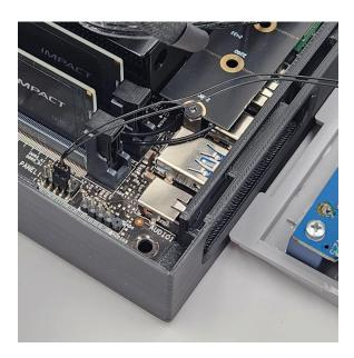
7. Set the front panel into its groove in the bottom shell.
