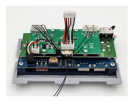
**7.** Plug the USB harness for the USB hub into the 4-pin USB hub header on the USB hub board.
