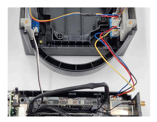
**14.** Start to slide the top shell onto the front panel from above. Check that the front panel reset switch lines up with the slot on the reset button.
