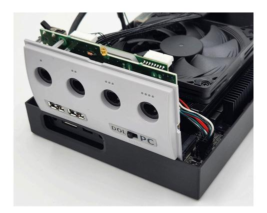
**8.** Place the power button standoff assembly inside the top shell and secure using (x2) M3 x 8mm thread-forming screws, tightening carefully.
