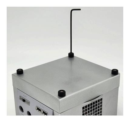
**Installing Wireless Antennas:** If the motherboard is equipped with a wireless module, install the wireless antennas onto the SMA connectors.
