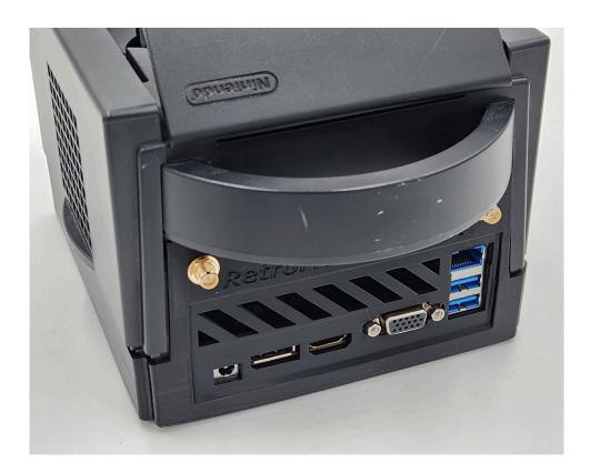
16. Ensure that the top shell is fully seated in the bottom shell around the perimeter. Check that no wires were pinched under the top shell mating lip, fell inside the CPU cooler fins, or are close to any of the system fan blades.
