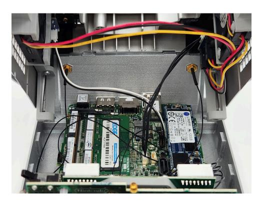
17. Check that the front panel reset switch lines up with the slot on the reset button.
