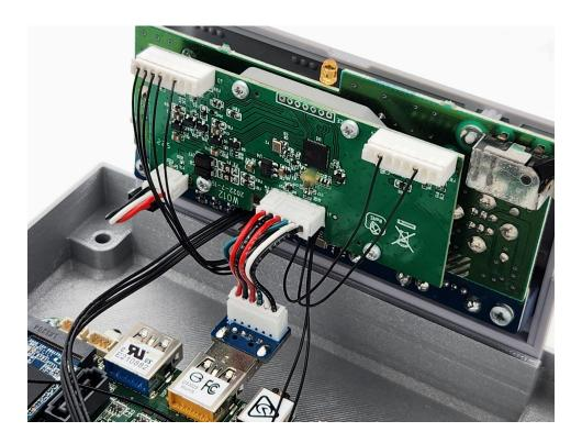
**9.** Plug the USB harness for the USB hub into the 4-pin USB header on the motherboard.
