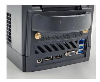
**17.** Secure the top shell to the bottom shell using (x4) M4 x 20mm bolts and (x4) rubber bumpers with the included 3mm hex key. Do not overtighten; the rubber bumpers should only be slightly compressed.
