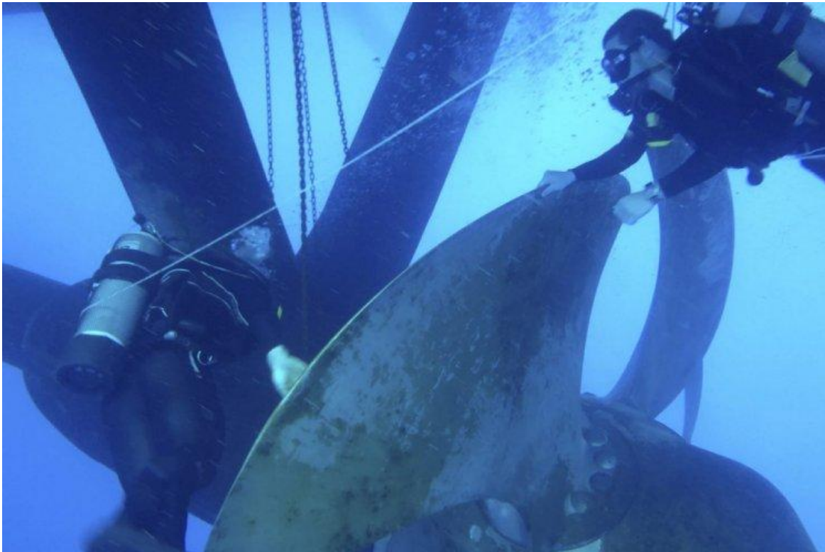
Able Seaman Marco Valensise and Able Seaman Michael McGuinness remove wire from HMAS Newcastle's main propeller shaft.
